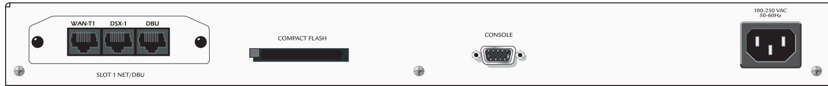
NETVANTA 1335 REAR PANEL LAYOUT
